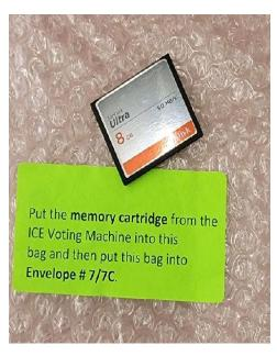
Serial # and Protective # are found at the Bottom of the End of Day Printout from the ICE machine just above the Signature lines. Public Counter is the number of votes cast on machine, this should match your poll book. Seal # is the red seal that goes back onto the cartridge door once the cartridge has been removed and put into the pink bubble bag.
